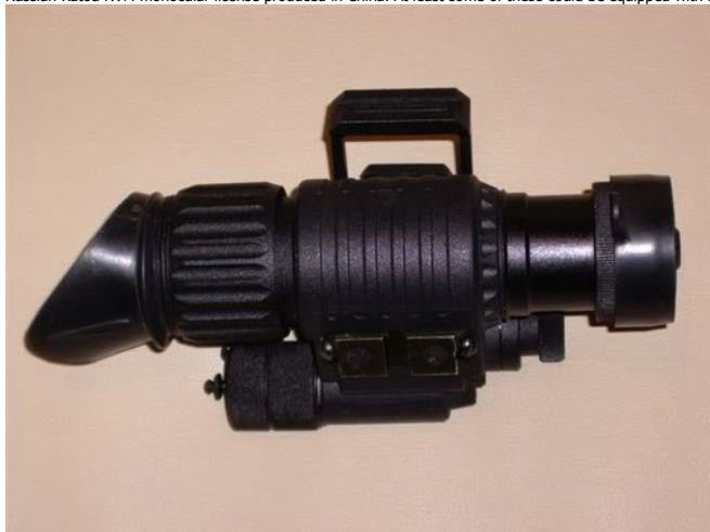
Russian Katod NVM monocular license produced in China. At least some of these could be equipped with Russian Gen3 tubes with 57-64 lp/mm resolution
