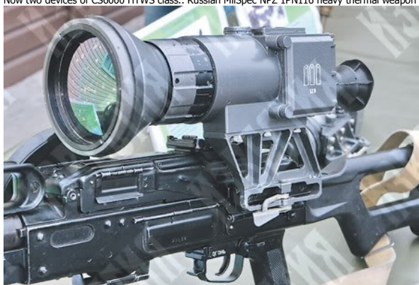
Now two devices of CS6000 HTWS class.. Russian MilSpec NPZ 1PN116 heavy thermal weapon sight and Chinese HTWS with 640x480 uncooled sensor mounted on their HSAI LR2A 50cal sniper rifle
