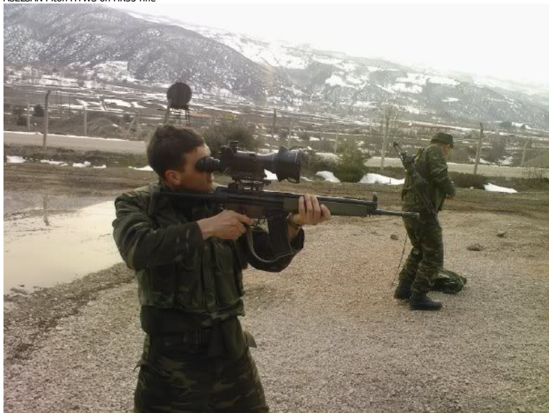
Polish thermal weapon sight CTS-1 by PCO corporation. The monocular on the last pic is 'Polish PVS-14' called PCO MU-3
