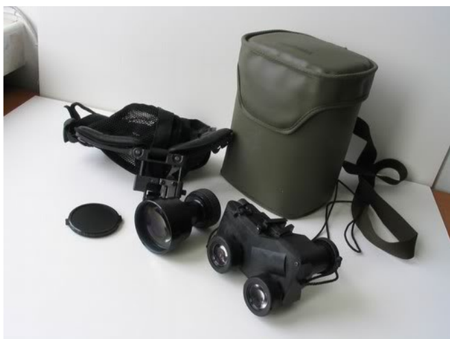
New generation of NVGs include LUCIE-NVT low profile goggles, originally a French design (Thales Angenieux), as well as BIM4 low profile monocular with integrated head-up display, similar to AN/PVS-21. (Swiss designed by Leica Vectronix). LUCIE is a standard goggle in French, Austrian and German armed forces.
