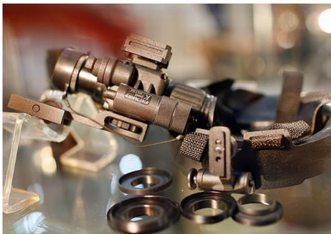
New generation of NVGs include LUCIE-NVT low profile goggles, originally a French design (Thales Angenieux), as well as BIM4 low profile monocular with integrated head-up display, similar to AN/PVS-21. (Swiss designed by Leica Vectronix). LUCIE is a standard goggle in French, Austrian and German armed forces.
