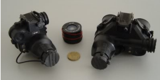
MonoKLARA and KLARA - size comparison. The tube in between is DEP XX2050 (XD-4)
